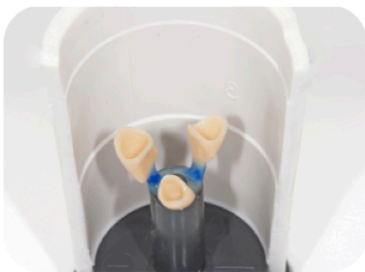
Simple spruing angulation for single units. Place sprue straight onto the incisal edge to avoid bubbles on the occlusion.
