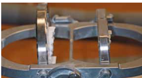
Fig. H The Eco milling machine can be set to different angles to mill every corner of the restoration.
