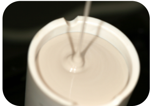
pour the investment between the upper line and the upper edge of the ring
