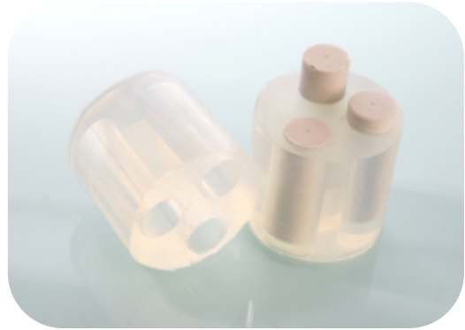
The plunger maker can be filled with the investment material used to invest the regular units. Make sure not to use high expansion ratios. A 50% expansion ratio for the press over porcelain and respectively the plungers are recommended.
