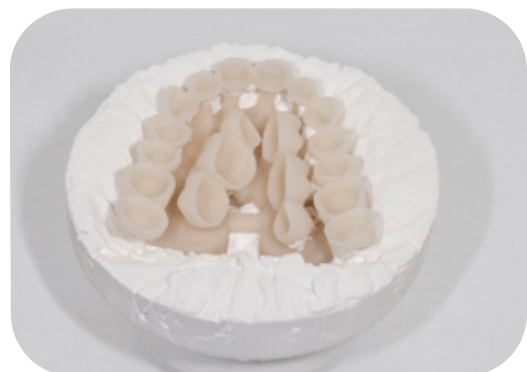
anteriors are pressed in dentin ingot for layering, posteriors in classic light ingot for staining
