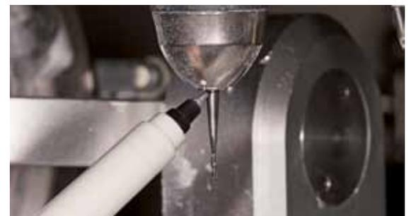
**Fig. F** For the "drop the pin" milling technique, the milling bur is dropped approximately 0.75 mm...
